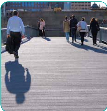
Southbank Pedestrian Bridge, Melbourne. Client – City of Melbourne. 745 m2 SISCO-Deck / 1398 L/M StructuralComp FRP Joist
