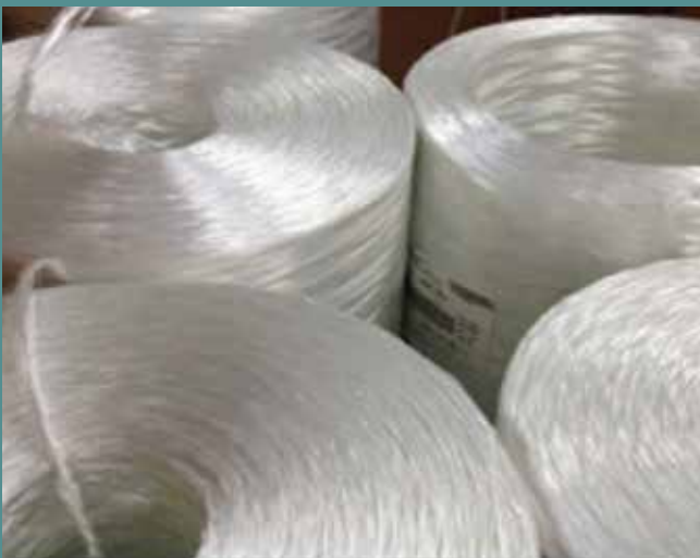
Rolls of glass fibers and an example of a glass fiber fabric comprising multiple fiber directions.
