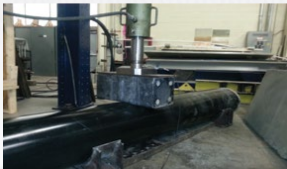
Crush Test on Concrete Filled Pile
