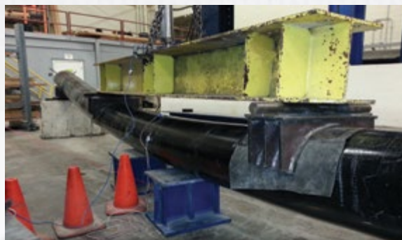
Full Section Testing of Concrete Filled Pile
