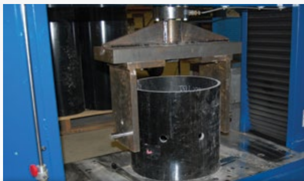
Bolted Connection Test - Parallel
