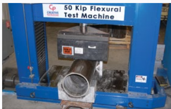
SUPERPILE® Crush Strength Test Set Up
